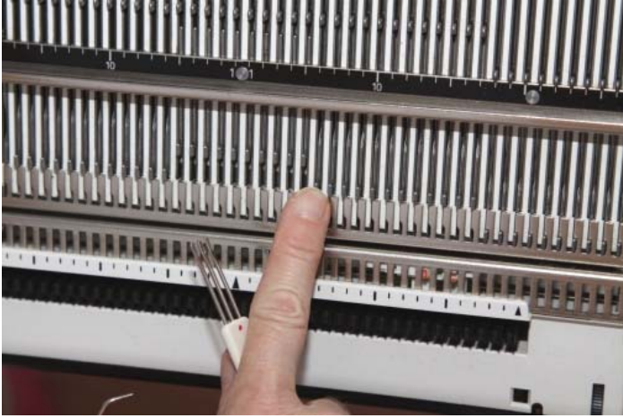
Figure 3: put first right-of -center pusher back into WP
